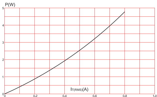
FIG.1: Maximum power dissipation versus RMS on-state current(full cycle)
